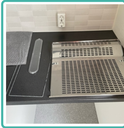
Clean and remove fat from grid and filter.
